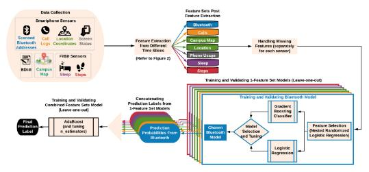
Fig. 1. Pipeline for the data processing and analysis.
